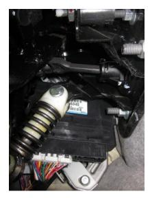
With the big booster out and arm for the MC unhooked grab its body and twist / pull it out.
