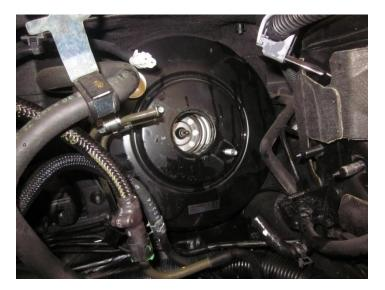
On the brake pedal you have to remove this pin that holds the brake booster fork.
