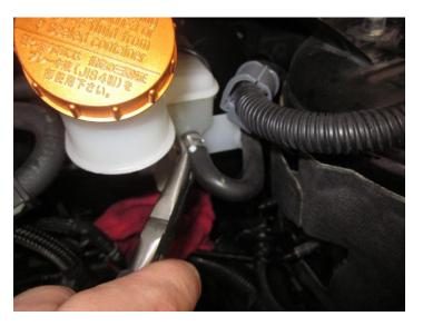
Pull and remove! Keep in mind brake fluid eats paint so any drips wipe off ASAP.
