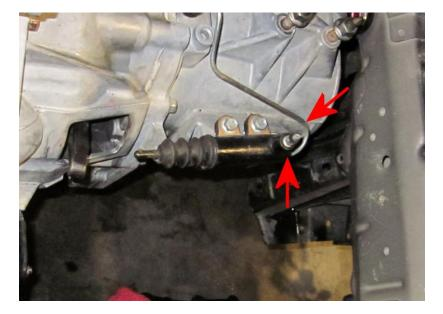
Loosen the bleeder and pump the clutch a few times then hold. Add fluid to the reservoir as needed and repeat until clutch is firm and actuating the slave as designed. If by chance the slave gets stuck use a screw driver to pry it back.
