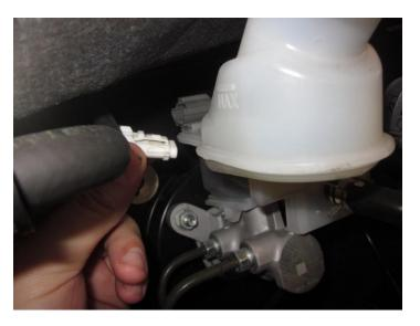
Now remove the hardline using a 12mm end wrench, you will have to get these pulled out of the way later.
