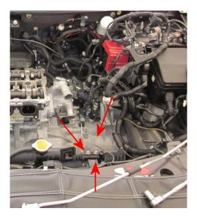
When you get to one of these clips pull firmly with vise grips or channel locks, then pull the line to you and up to remove line from bracket.
