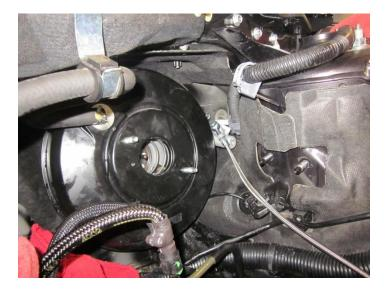
Now that the brake booster is back on its time to go put its 4 bolts and pin back in as well as get the MC arm secured to the clutch pedal. You know that weird little "L" shaped piece; here's what it's for. Slide it over the ball and cinch it down.
